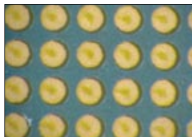
Figure 4 - 37.5 \mu m solder mask clearance, exposed with conventional printer
