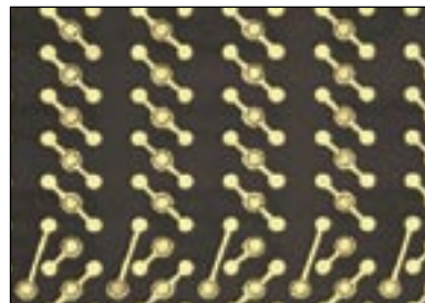
Figure 2 - Sequential build-up board with 35 \mu m annular ring
