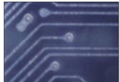
Figure 3 - 125 \mu m pads over 75 \mu m via holes (25 \mu m annular ring)
