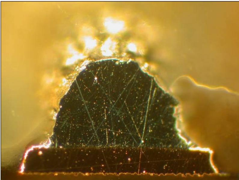
Figure 4 – Cross-section of an acceptable solder joint and surface graping
