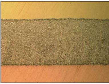
*Figure 5 - Cross-section of a large-crystalline grain structured solder joint*
