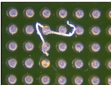
Figure 1 – Fibre caught in BGA print Figure 2 – Contaminated stencil apertures
