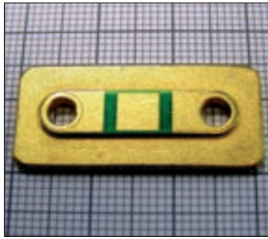
Figure 5 - HF circuit board with bonded Cu coin
