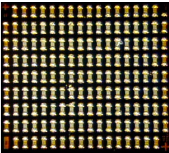
Figure 3 – The difference in the relative number of voids under the chip when a small amount of standard electronics resin and curative mixture was applied, observed through the glass slide, after the solder reflow
