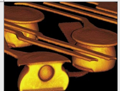
3D CT of CSP solder joints
