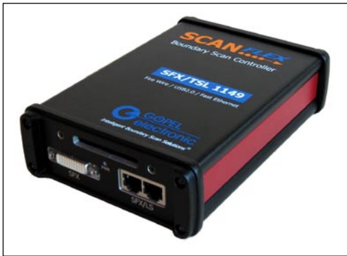
Figure 4 – Hardware – Boundary Scan Controller from GOEPEL electronic (SFX-TSL1149.x)
