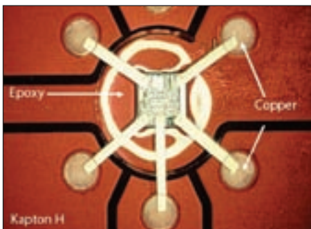
Figure 6 - Direct die attach. M 3 D deposited Ag interconnects from the smart card contact pad over epoxy adhesive and connection to the IC. Line width approximately 150 microns
