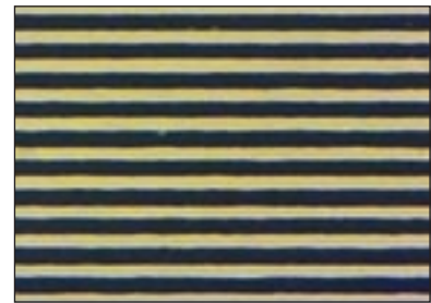
Figure 2 - 10 micron Ag lines on glass. Note smooth surface and high edge definition
