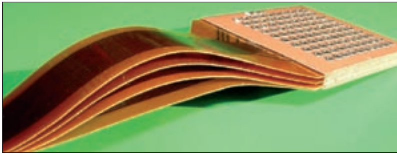
Figure 7 - Multiflex board with non-bonded flexible area
