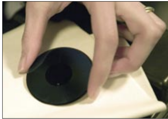
Figure 4 - An imprinted 2-inch wafer
