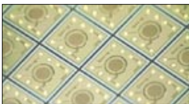
Figure 1 - MEMS microphones within 6-inch wafer, close-up
