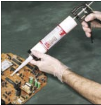
Figure 4 - Thermally conductive pastes make it easier to disassemble components
