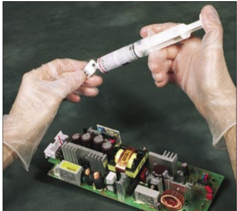
Figure 1 - Heat transfer compounds can be silicone or non-silicone based
