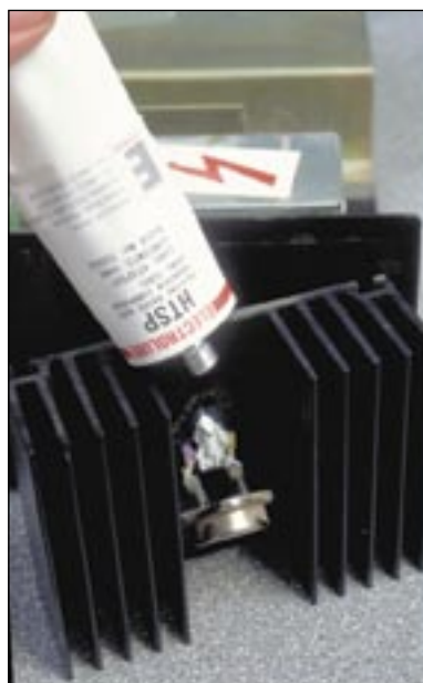
Figure 3 - Silicone-based pastes often have higher operating temperatures than their non-silicone alternatives
